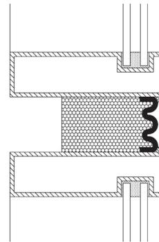
Seismic Colorseal is uniquely suited to sealing structural joints in curtain walls. Non-invasive anchoring means that mullions are not violated by screwing through them as occurs with "strip-seal" systems.
