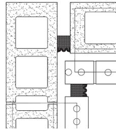
Seismic Colorseal is an excellent, simple sealing solution at inside corner conditions where it is impossible to install mechanically fastened 'strip-seal' systems. In cavity-wall conditions, installation of Seismic Colorseal in the structural backup maintains integrity of thermal insulation as well as the air barrier while preventing passage of cavity moisture into the structure.
