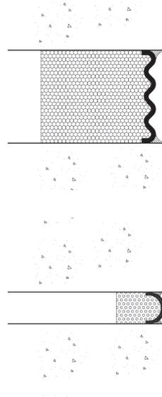
Seismic Colorseal is held in place by the back-pressure of the expanding foam in conjunction with a field-installed bead of silicone caulk at the substrate-to-bellows interface.
